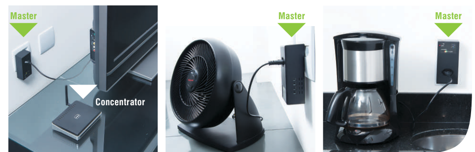
Appliances' metering whit smart plugs and communication's concentrator
